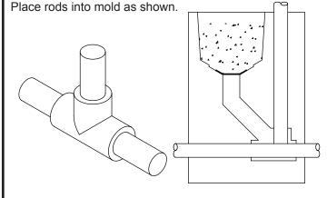
Place rod into mold as shown. With RR-14 molds, rods are uncut.
